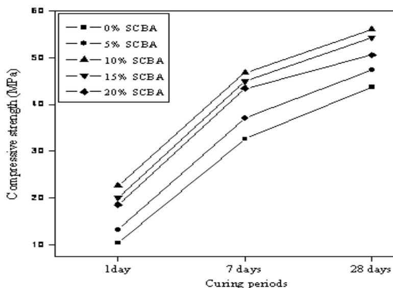
Fig. 1. The compressive strength of OPC and OPC + 10% SCBA.
