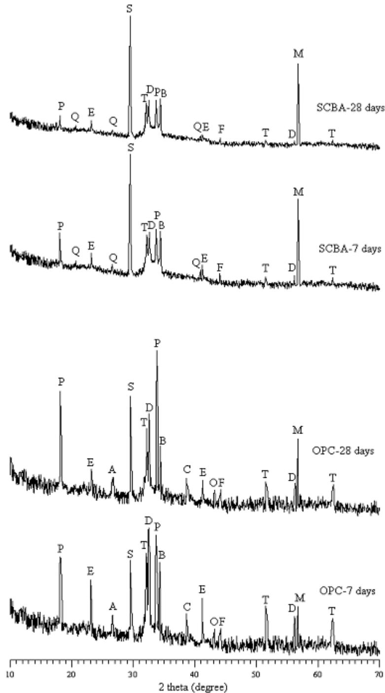
Fig.2. The XRD spectra of hydrated OPC and OPC + 10% SCBA paste at 7 days and 28 days
