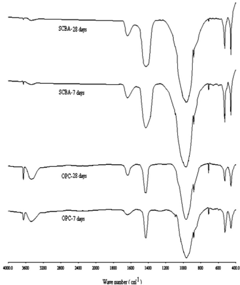
Fig.3. The FTIR spectra of hydrated OPC and OPC + 10% SCBA paste at 7 days and 28 days
