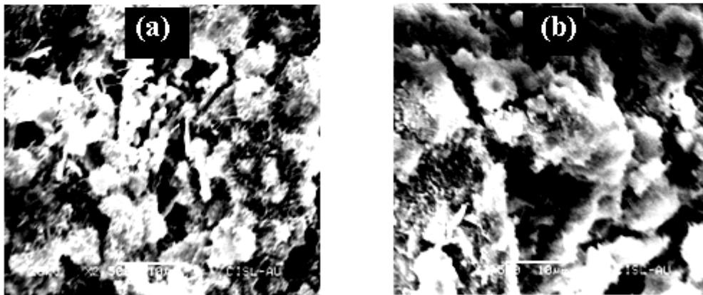
Fig.5. The SEM micrographs of OPC + 10% SCBA ( $\times 2500$ )
