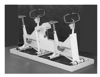
Figure 1: Tandem-bicycle ergometer
