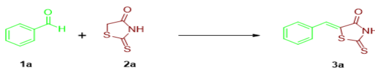
Figure 1: Synthesis of 5-Arylidene-rhodanine derivatives 3a by using DIPEAc as RTIL.
