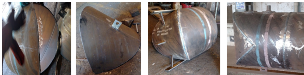
Figure 1: (Sequence left to right): Female part, male part, female and male part welded together, female and male part welded to the pipe
