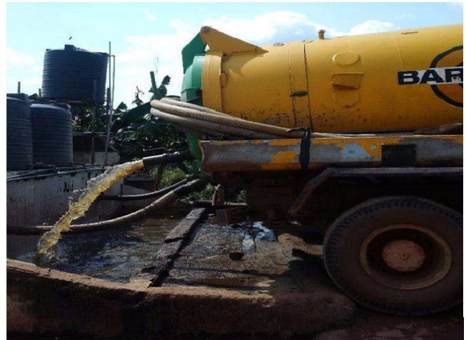
Figure 1: Modern Sludge management techniques used by developed nations (left) and vacuum trucks used to empty pit latrines and septic tanks used in developing countries (right).
