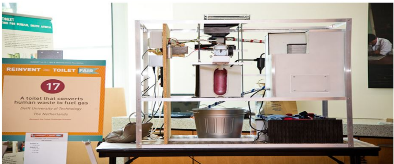
Figure 5: The plasma gasification reactor.
