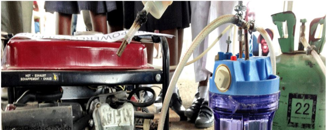
Figure 4: Generator that uses urine as fuel.
