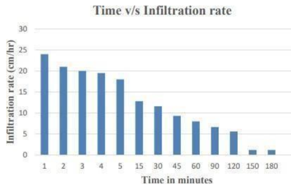
Figure 15. Determination of infiltration rate of soil
