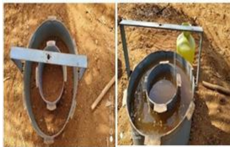
Figure 3. Installation of Double Ring Infiltrometer
