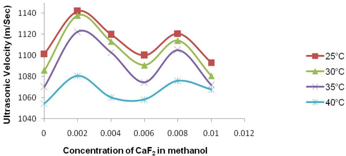
Figure 3. Variation of ultrasonic velocity with a concentration of CaF<sub>2</sub> in methanol
