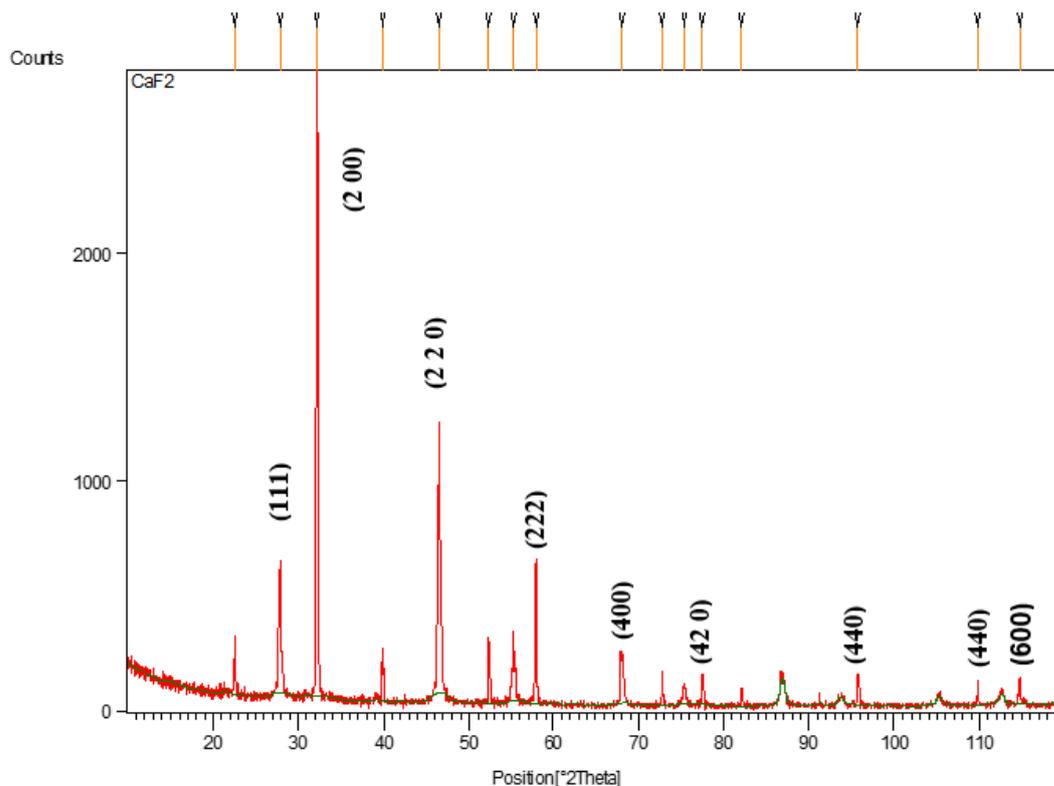
Figure 1. X-ray Diffraction pattern of  $\text{CaF}_2$
