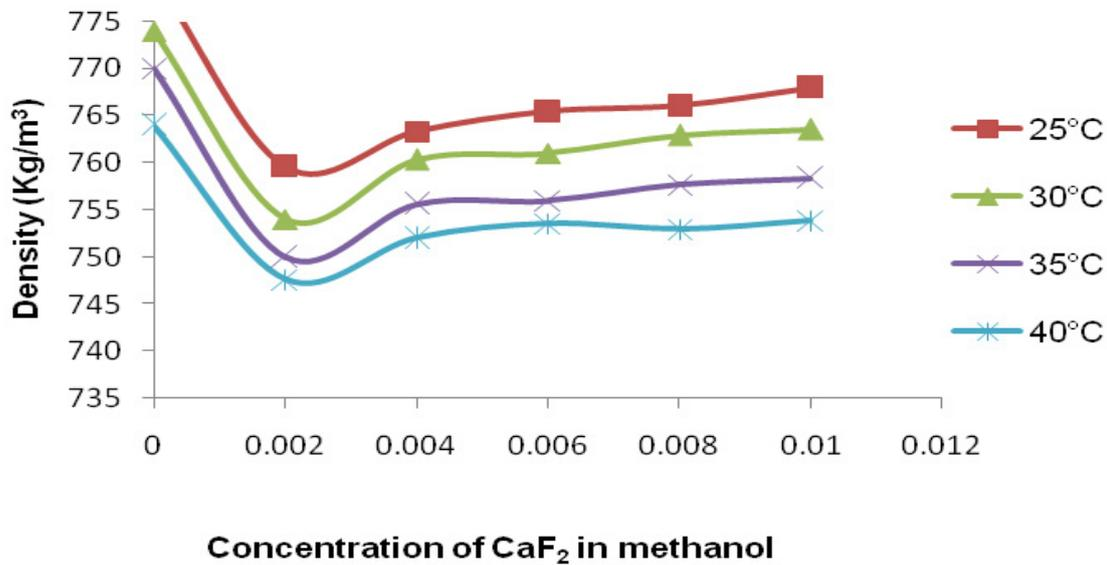
Figure 4. Variation of density with a concentration of CaF<sub>2</sub> in methanol
