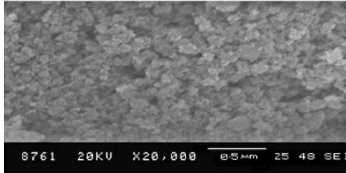
Figure 2. SEM images of synthesized  $\text{CaF}_2$
