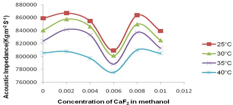
Figure 9. Variation of acoustic impedance with concentration of CaF<sub>2</sub> in methanol
