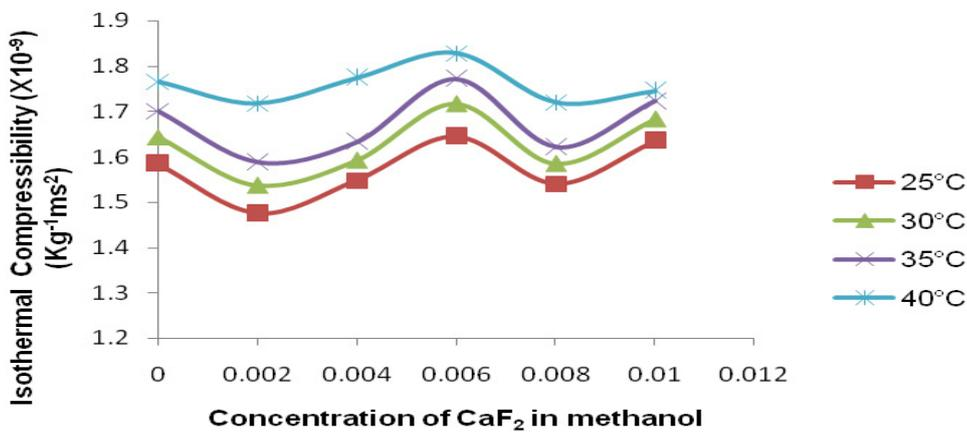
Figure 6. Variation of isothermal compressibility with concentration of CaF<sub>2</sub> in methanol
